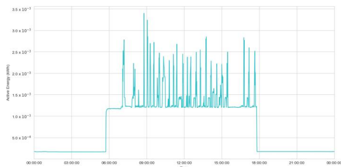
Fig. 1: Line graph displaying the active energy during a treatment day at the SWWCC. Times of interest include linac engineers' run-up at 07:00, radiographers' QC at 07:50, DIBH treatment at 10:15 and SGRT staff training at 15:30.
